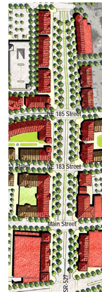
FIG. 2.8 ILLUSTRATIVE PLAN VIEW OF ENVISIONED MULTIWAY BOULEVARD AND ITS FRONTING MIXED-USE DEVELOPMENT WITH GROUND-FLOOR RETAIL
