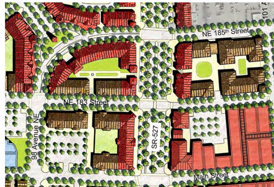
FIG. 2.29 ILLUSTRATIVE PLAN VIEW OF ENVISIONED 98 TH AVENUE NE TO NE 185 TH STREET CURVED STREET CONNECTOR WITH SURROUNDING MIXED-USE DEVELOPMENT
